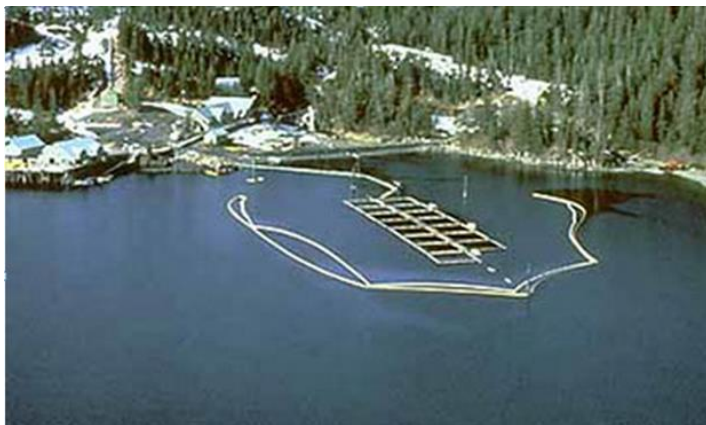
Figure 6.2 Boom surrounding a set of floating pens at a salmon hatchery in Prince William Sound, AK, to protect the pens from oil spilled from the Exxon Valdez tanker. Source: NOAA
