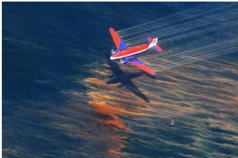
Figure 6.20 An aircraft releases chemical dispersant over an oil slick in the Gulf of Mexico in 2010. Source: NOAA /US Coast Guard
