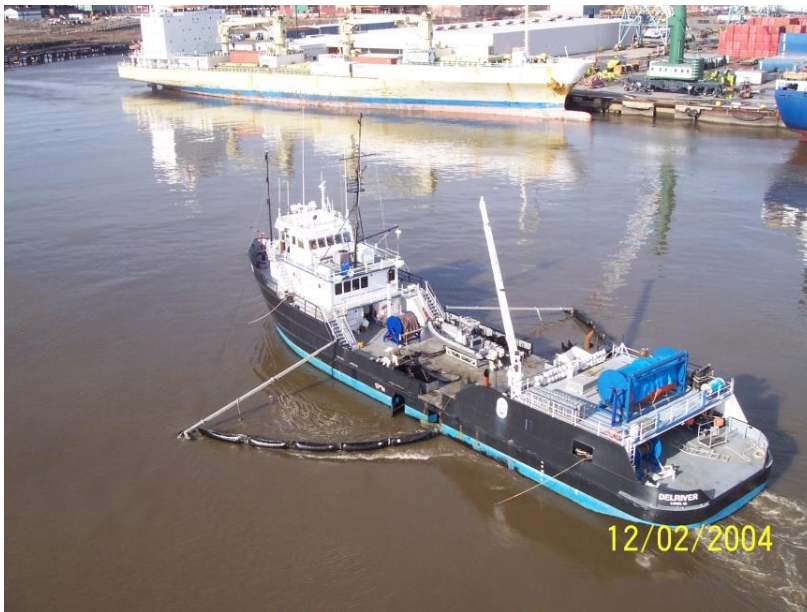
Figure 6.4 Skimming the Delaware River in Philadelphia following the M/T Athos I spill on November 26, 2004. Source: NOAA.
